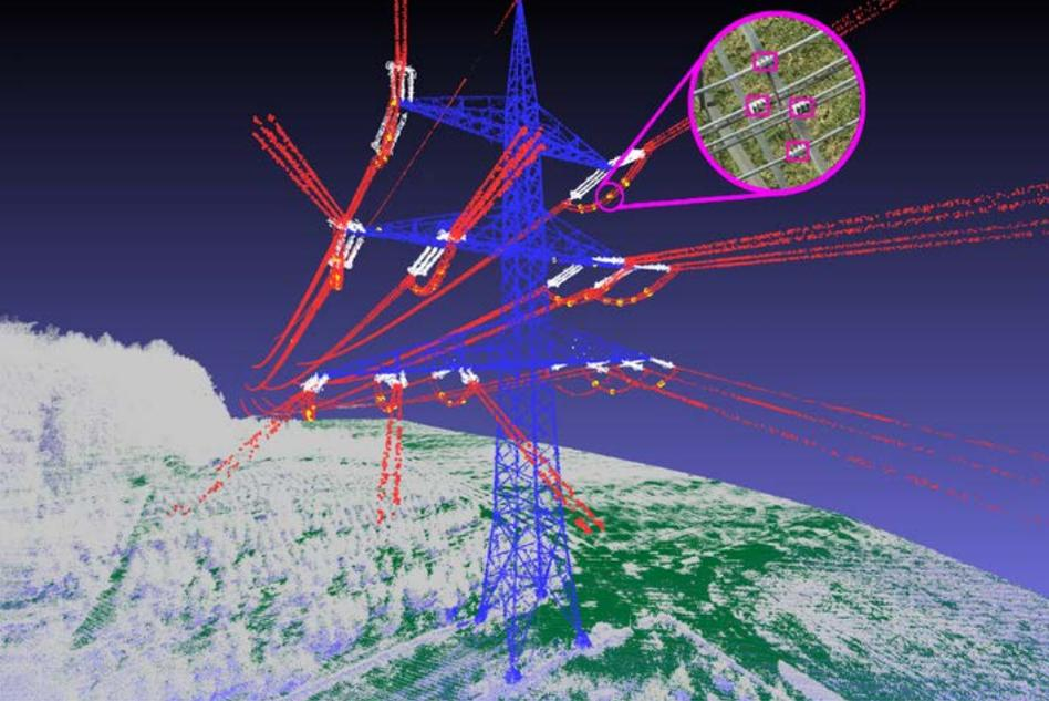
**Automatic inventory system for clamping connections for thermal inspections, illustration: Siemens AG Austria**
